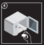
Place the tablet on the grill in the middle of the oven chamber.
